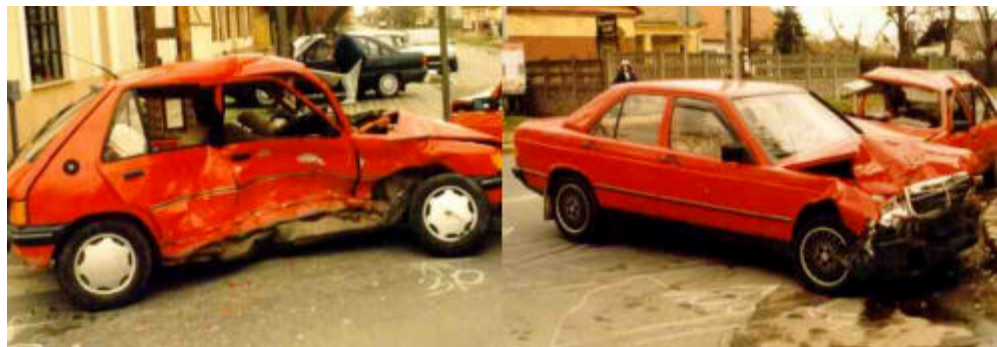
Figure 12 – Impact at the sill beam height
