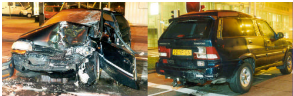
Figure 21 – The front of a small passenger car that drove into the back of a SUV.
