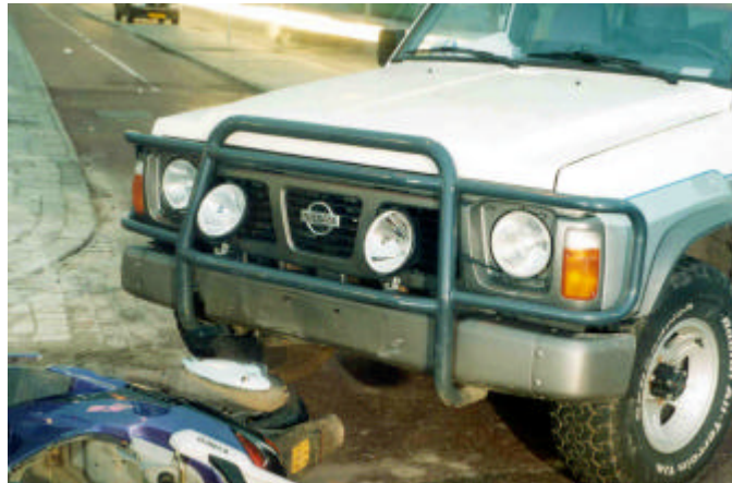
Figure 14 – Example of a pointed construction
