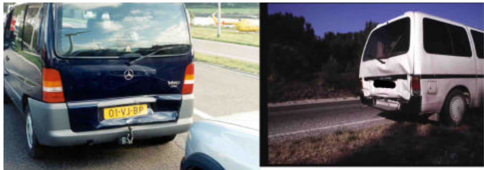
Figure 10 – Deformation of the rear door of a small van
