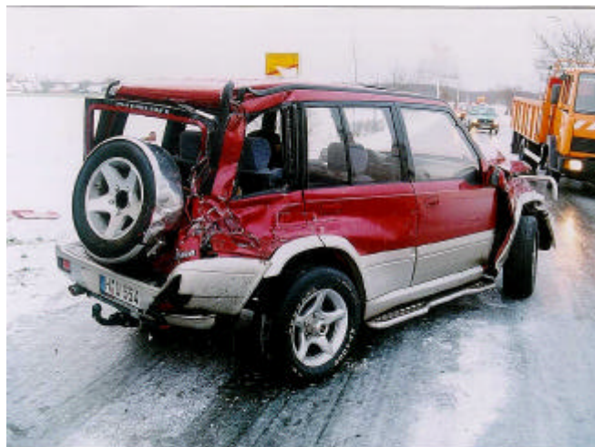
Figure 17 – Rear door deformation due to the spare wheel position
