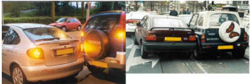
Figure 7 – Comparison of the bumper height between a small SUV and a passenger car
