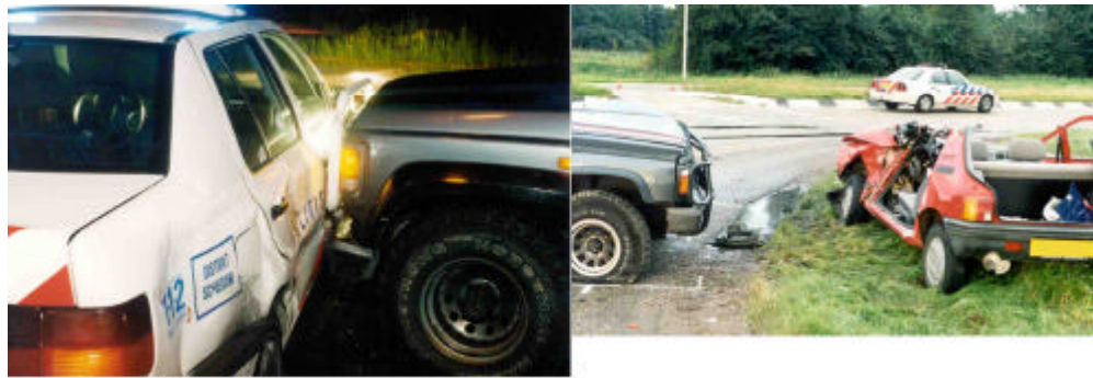
Figure 11 – Impact much higher than the sill beam height, without any bull-bar deformation
