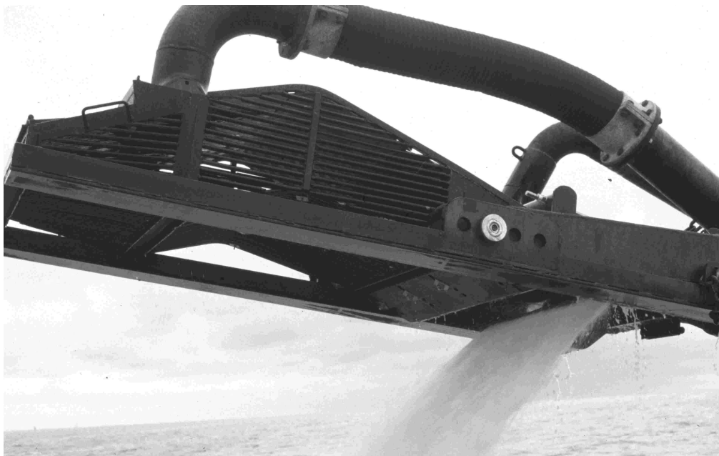
Figure 16: Close-up of a suction dredge. Photo Jaap de Vlas.
