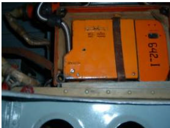
Fig 4. FDR unit with cover removed, consisting of recording unit (left) and tape cartridge (right)
