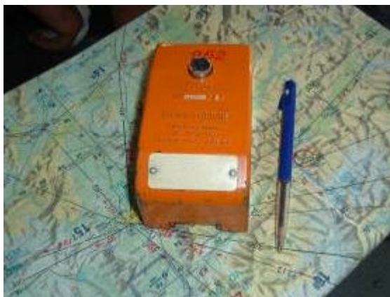
Fig 5. FDR tape cartridge (sample of the two recovered units)
