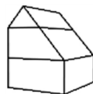
S3 - Woning 3-laags mank dak
