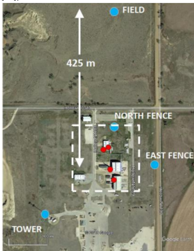
Figure 5.1 Top view of the release locations (red circles) and concentration monitors (blue circles) at the Balko compressor station (image copied from [25]).
