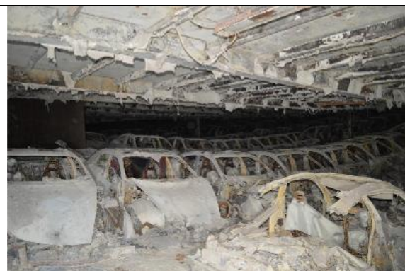
FIGURE 10A: 9 TH DECK BURNED CARS (Source: Physical inspection O/B - Fire Expert Report)
