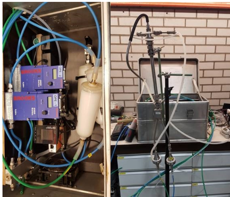
Figure 3: Measurement set up for measurement of particulate matter gravimetrically. Left: mass flow controllers for a stable sample flow and dilution. Right: filter holders.
