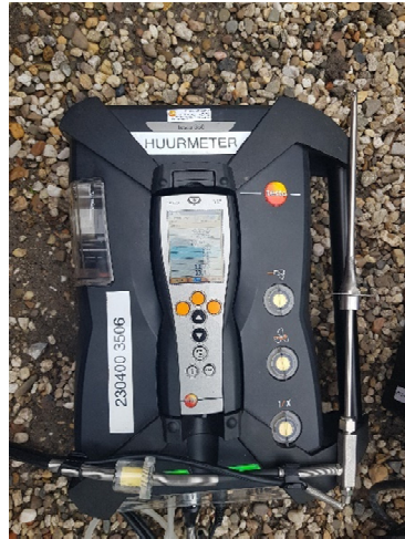
Figure 2: Testo 350 gas analyser used for the measurement of gas concentrations NO, NO 2 , O 2 , CO, C x H y and CO 2 (from O 2 ) in the exhaust of stationary machines at a construction site.
