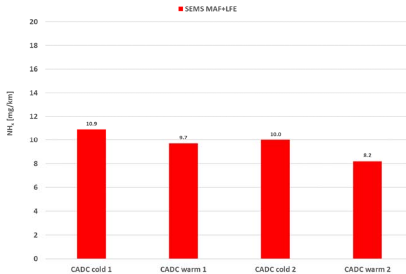
Figure 11-4: NH 3 CADC test results with cold and warm starts of the VW Polo Euro 6 petrol measured with MEMS (MAF + LFE based).
