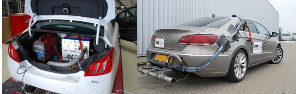
Figure 3 Portable Emission Measurement System (PEMS)
