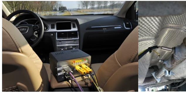
Figure 4 Smart Emission Measurement System (SEMS)
