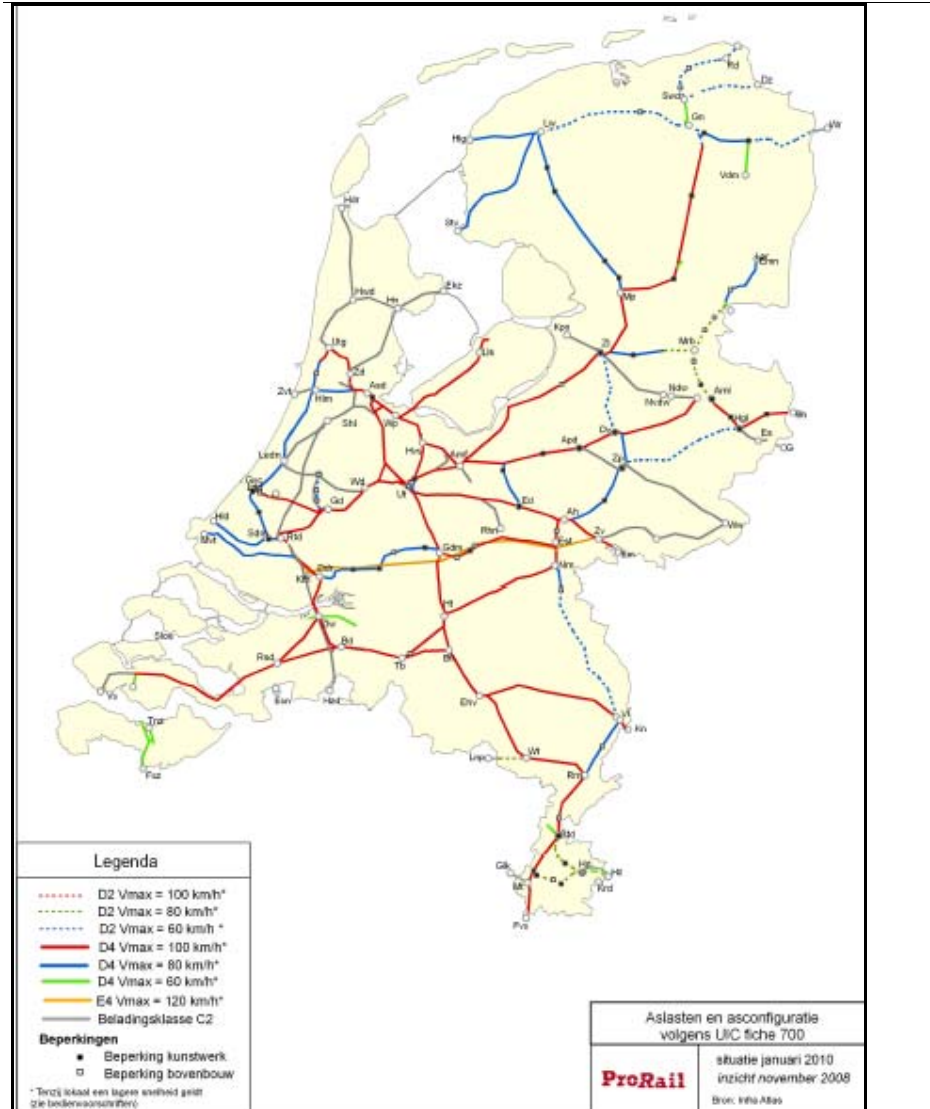
Figure 4.9 Axis loads and maximum speed in the Netherlands
