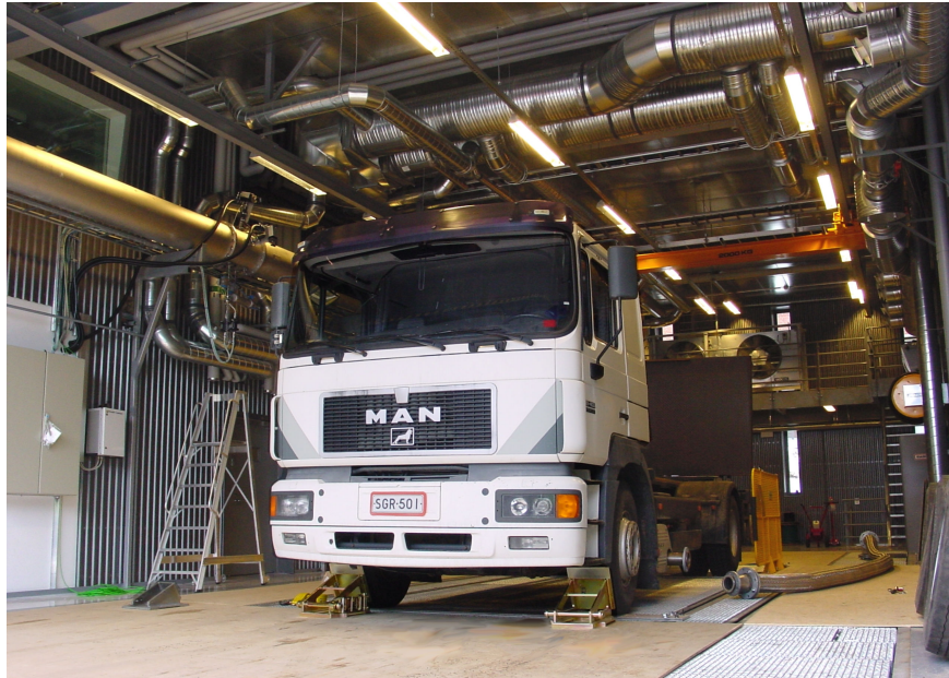
Figure 4: Chassis dynamometer test cell (vehicle shown was not used for the test programme)
