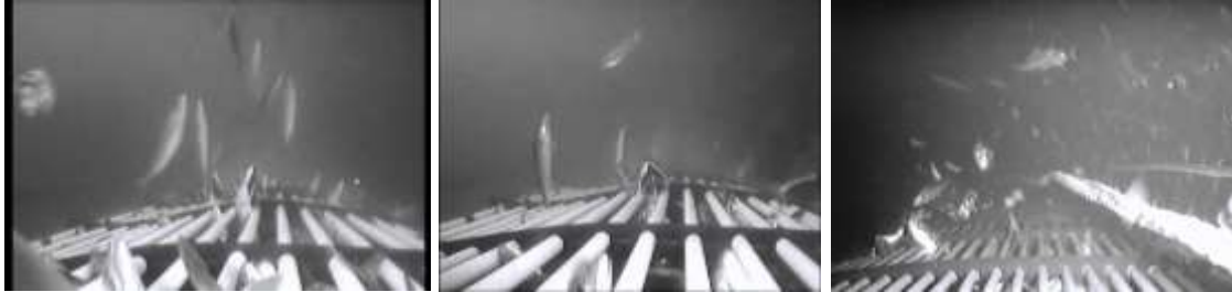
Figure 4.9. Camera footage from the gear adaptation with flexible tubes (left and middle mackerel, right herring)
