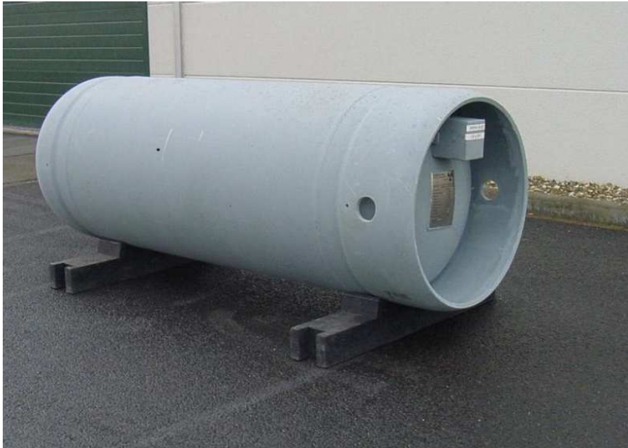
Figure 1-3 Standard 30B UF 6 cylinder
