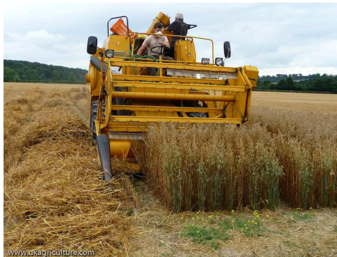
Figure 2: Combine harvesting of oats. Straw is left to dry in the field (left hand side of picture). Source: UK Agriculture
