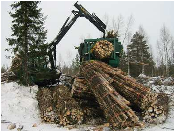
Figure 10: Forest residue bundles and bundling machine. Source: Northern Woodheat [Source: http://elearn.ncp.fi/materiaali/kainulainens/nwh/woodfuel_supply_chains/forest_chips/bundling.htm ]
