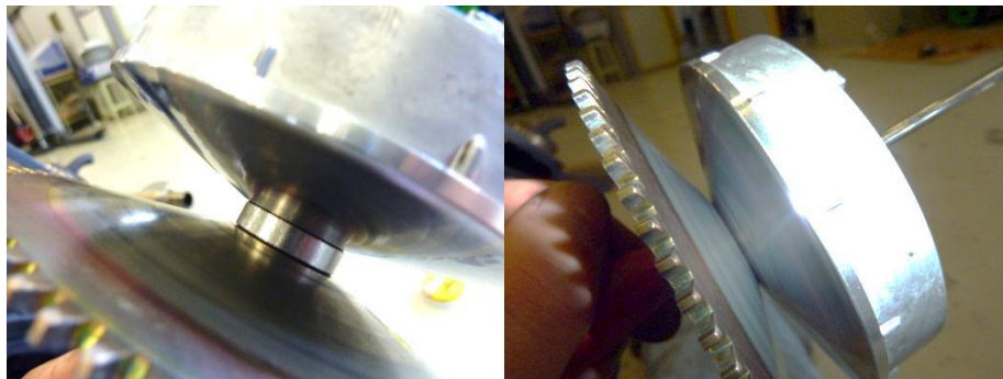
Figure 1: Variomatic with (left) and without (right) ring
