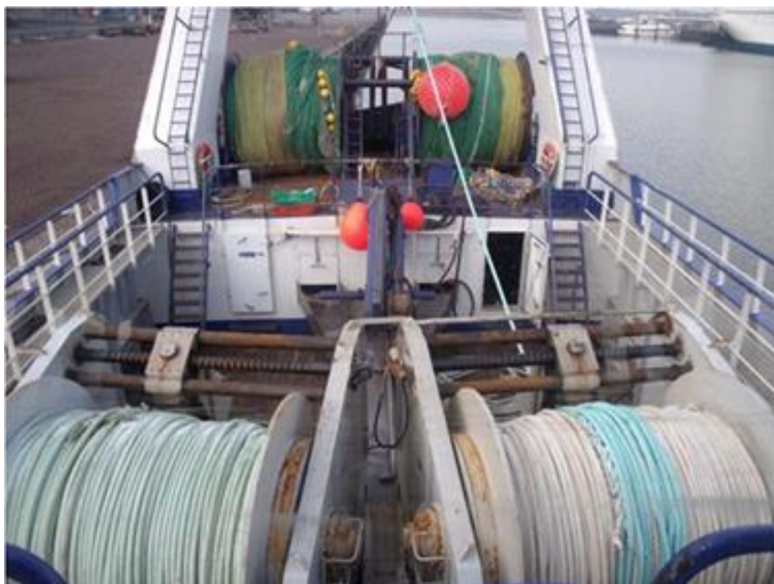
Figure 33: Stern trawl gear on the net drums
