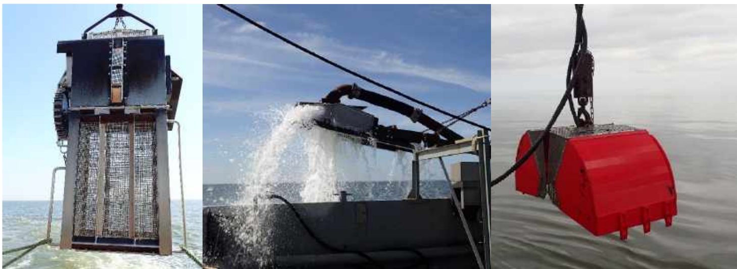
Figure 3.5. Trawled dredge (left), modified hydraulic dredge (middle) and hydraulic grab(right) (Photographers: Karin Troost and Jack Perdon).
