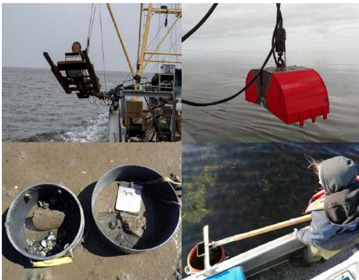
Figure 3.3. : “Stempelkor” (top left), hydraulic grab (top right), corer with sieve (bottom left) and cockle-sampling device (Photographers: Karin Troost, Douwe van den Ende and Herman Troost).
